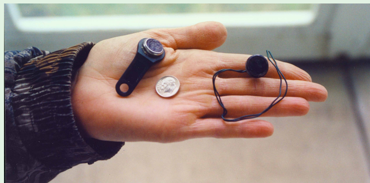
▲ A data logger used in the Incubation Rhythm Study.
